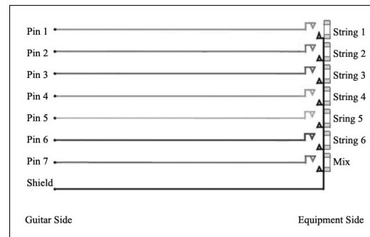
Figure 2. 13-pin Breakout Box Schematic[4]
